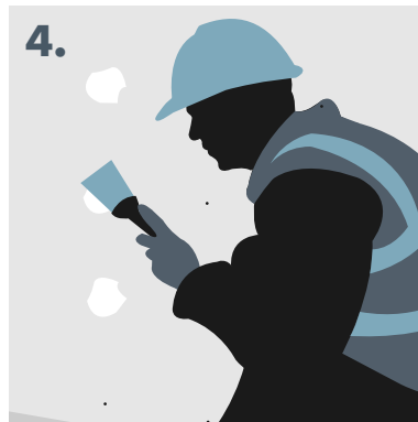
4. Covering screw heads with Knauf Aquapanel Exterior Joint Filler - Grey.
