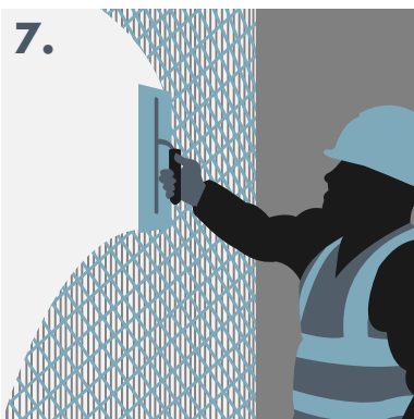
7. Covering mesh with basecoat.
