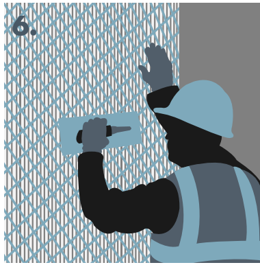
6. Applying reinforcing mesh.
